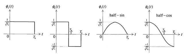
It can be verified that  $\phi_1(t)$  and  $\phi_2(t)$  forms a set of *orthonormal* basis functions. Clearly list three other pairs of *orthogonal* functions.
