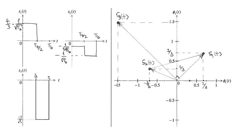
[2] (c) Next, consider signal  $s_3(t)$  as shown above. It is known that  $s_3(t)$  can also be represented as a linear combination of  $\phi_1(t)$  and  $\phi_2(t)$ . Obtain such a combination and clearly show the location of  $s_3(t)$  on the same signal space diagram in Part (b).
